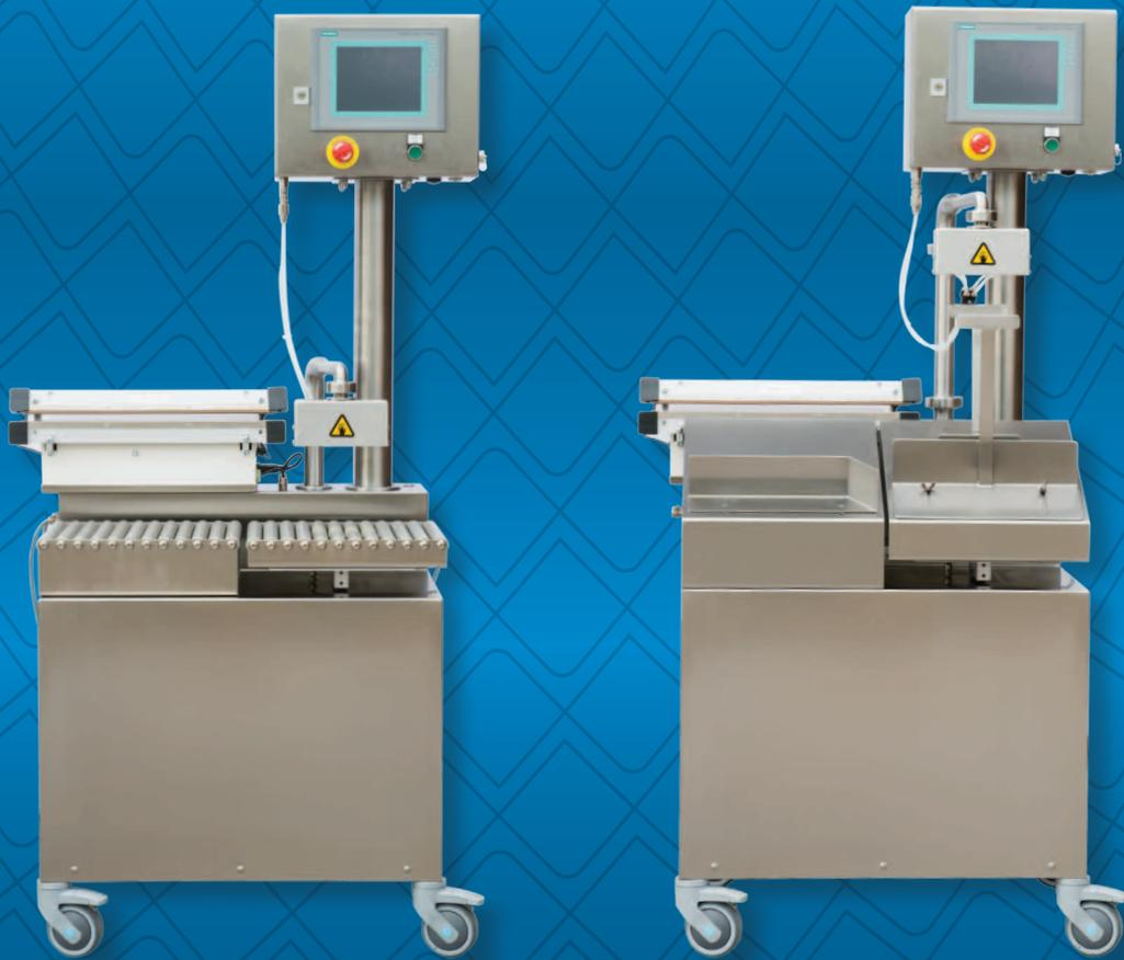
The **HOT-FILL DOS 2** ensures quick and precise dispensing of liquid food products. Soups, sauces and mashed potatoes are filled into bags and containers effortlessly. The built-in scale ensures that weighing of the product happens in one and the same workflow saving time in the kitchen. Changing the filling process from bags to containers only takes a few moments. Simply remove the bag holder, fit the roller track and the HOT- FILL DOS 2 is ready.
